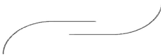
Gambar 2. 5 Rotor *Savonius* Dua Bucket “L” Dengan Overlap
