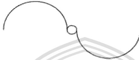
Gambar 2. 3 Rotor *Savonius* Dua Bucket Tanpa Overlap
